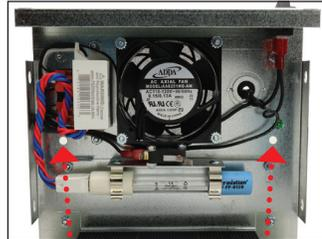
Photo 3: Mounting bracket holes (hardware provided)
