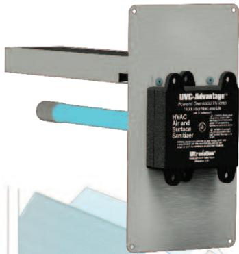
UVC-Advantage PCO can be installed near the HVAC cooling coil where its germicidal UV light will disinfect the wet coil and surrounding parts. If needed, a second UV light for disinfection can be installed and easily connected to the purifier for power with an adapter accessory.
